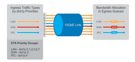
ETS uses the following traffic groupings to select multiprotocol traffic for transmission:
