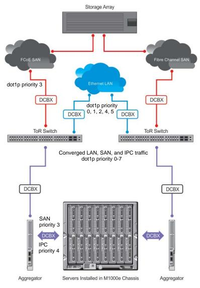
**QoS Traffic Classification**: On the Aggregator, the service-class dynamic dot1p command has been used in Global Configuration mode to map ingress dot1p frames to the queues shown in Table 6-6. For more information, refer to QoS dot1p Traffic Classification and Queue Assignment.
