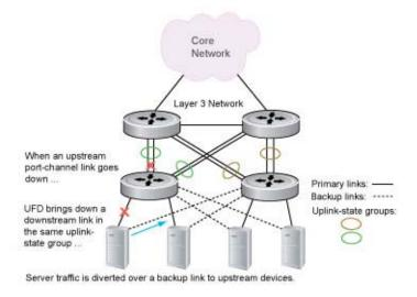
If only one of the upstream interfaces in an uplink-state group goes down, a specified number of downstream ports associated with the upstream interface are put into a link-down state. This number is user-configurable and is calculated by the ratio of upstream port bandwidth to downstream port bandwidth in the same uplink-state group. This calculation ensures that there are no traffic drops due to insufficient bandwidth on the upstream links to the routers/switches.
