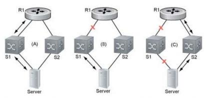
A: Switches1 and 2 have upstream and downstream connections to Router1 and Server via primary links. B; Upstream link between Switch1 and Router1 fails. Downstream link with Server stays up temporarily. C: Switch1 disables downstream link to Server. Server starts to connect with Router1 using backup link to Switch2; Switch2 starts to use the backup link to Router1.
