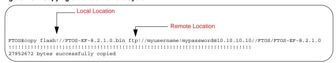
Figure 4-10 shows an example of using the copy command to import a file to the Dell Force 10 system from an FTP server.
