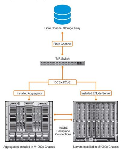
In Figure 8-11, DCBX and PFC are enabled on the Aggregator (FIP snooping bridge) and on the FCF ToR switch. On the FIP snooping bridge, DCBX is configured as follows:
