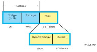
TLVs are encapsulated in a frame called an LLDP data unit (LLDPDU) (Figure 14-2), which is transmitted from one LLDP-enabled device to its LLDP-enabled neighbors. LLDP is a one-way protocol. LLDP-enabled devices (LLDP agents) can transmit and/or receive advertisements, but they cannot solicit and do not respond to advertisements.
