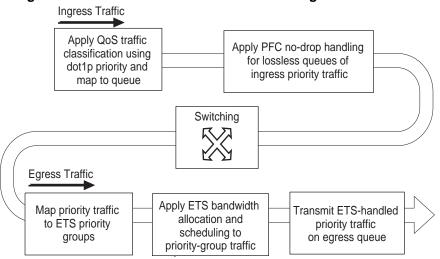
Figure 6-3. DCB PFC and ETS Traffic Handling
